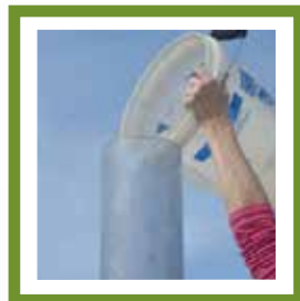
Figure 9: Filling Infiltrator with Water
