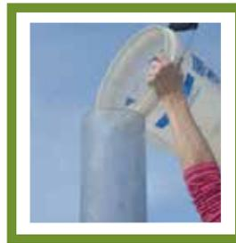
Figure 9: Filling Infiltrometer with Water
