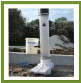
Figure 7: Infiltrometer Placement
